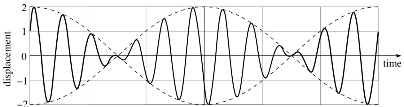
The displacement – time graph of this superposition of signals is shown in Figure for the case where the two equal amplitude original oscillations have frequencies in the ratio  $13 : 11$ .
