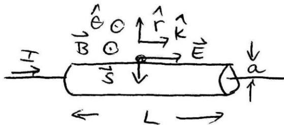
Because the Poynting vector points radially inward we only calculate the flux over the cylindrical body of the resistor. Hence we set  $r = a$  for Poynting vector and then integrate it over the outside cylindrical area of the resistor. For a closed surface we choose  $\hat{n}_{out} = \hat{r}$  and so  $\vec{S}\hat{r} = -|\vec{S}|$ .
