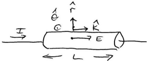
There is an electric potential difference across the resistor that is equal to  $\Delta V = IR$ . The electric field is uniform in the resistor so  $|\Delta V| = |\int \vec{E} d\vec{s}| = EL = IR$ . Therefore the direction and magnitude of the electric field is given by
