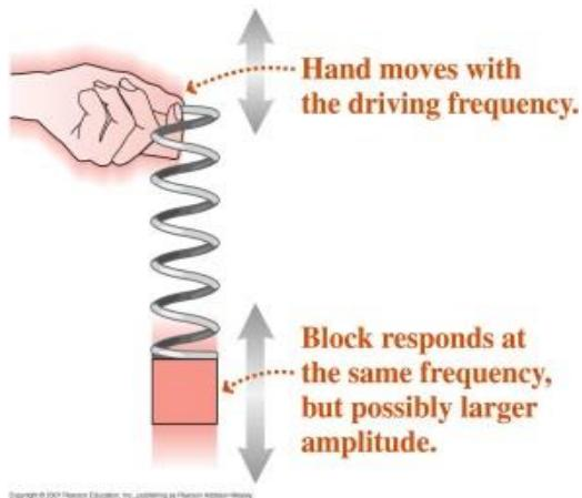
For example, in the case of the (vertical) mass on a spring the driving force might be applied by having an external force ( $F$ ) move the support of the spring up and down. In this case the equation of motion of the mass is given by,
