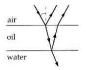
Since 1<1.45, the light reflected from the top of the oil film undergoes phase reversal. The light reflected from the bottom undergoes no reversal because 1.45>1.33.
