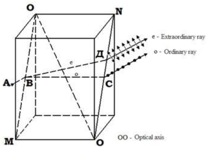
In uniaxial crystals in the same direction, called the optical axis, along which the distribution is no distinction between ordinary and extraordinary rays. Any line parallel to the direction of the optical axis will also be the optical axis. Any plane passing through the optical axis and the incident beam, called the principal or main section of the crystal planes.
