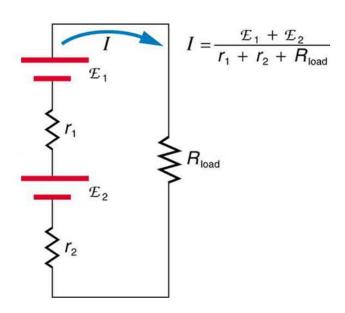
$$I_1 = \frac{E_1 + E_2}{r_1 + r_2 + R} = 3 \text{ A}$$
