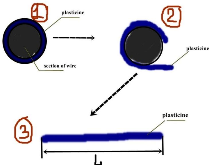
Look at this picture. Step 1: take a wire and stick it by a plasticine as shown in figure 1 (not necessarily all wire only part, but on all sides).
