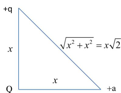
$$U = k_e \left( \frac{Qa}{x} + \frac{Qq}{x} + \frac{qa}{\sqrt{2}x} \right) = \frac{k_e}{x} \left( Q(a+q) + \frac{qa}{\sqrt{2}} \right) = 0$$
