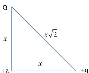
$$U = k_e \left( \frac{Qa}{x} + \frac{aq}{x} + \frac{qQ}{\sqrt{2}x} \right) = \frac{k_e}{\sqrt{2}x} \left( Q(\sqrt{2}a+q) + \sqrt{2}qa \right) = 0$$
