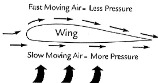
During flight air naturally flows over and beneath the wing and is deflected upwards over the top surface and downwards beneath the lower surface. Any difference in deflection causes a difference in air pressure ('pressure gradient') and because of the airfoil shape the pressure of the deflected air is lower above the airfoil than below it. As a result the wing is 'pushed' upwards by the higher pressure beneath or, you can argue, it is 'sucked' upwards by the lower pressure above.
