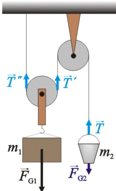
The force equation for movable pulley is
