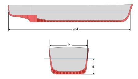
Let's consider a ship that moves from salt water of density  $1015\frac{kg}{m^3}$  to salt water of density  $1025\frac{kg}{m^3}$ . The ship must displace the same mass of water in each case. The mass of water displaced in case of salt water with density  $1015\frac{kg}{m^3}$  will be:
