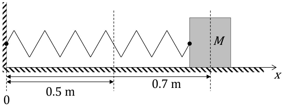
Since the force of 25.6 N is required to maintain the spring stretched by the length of 0.2 m, the stiffness of the string has the following value
