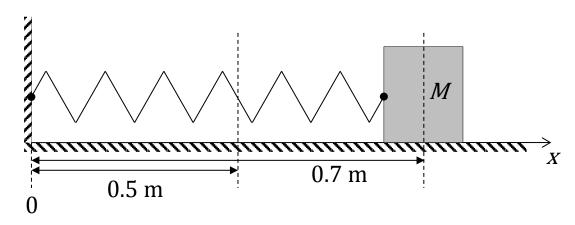
Since the force of 25.6 N is required to maintain the spring stretched by the length of 0.2 m, the stiffness of the string has the following value
