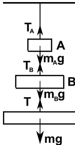
Let's draw a free-body diagram. From the diagram we can see that  $T_A + T_B + T - m_A g - m_B g - mg = 0$ . Because the balances A and B are massless, the tension on the each spring will be the same. Therefore,  $T_A = T_B = T$ ,  $m_A = m_B = m = 2\text{kg}$ .
