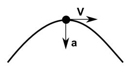
When particle going ground a curve, the acceleration will be directed toward the center of a curve. The acceleration in this case would be:
