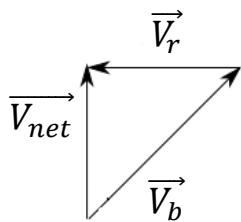
Let the  $\vec{V}_b$  is the boat speed in still water,  $\vec{V}_r$  is the speed of river and  $\vec{V}_{net}$  is the net speed of the boat, and let us build the vector diagram. In order to find  $\vec{V}_{net}$  we apply the Pythagorean theorem:
