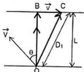
Suppose the boat starts in travelling in a direction making an angle  $\theta$  with OB as shown in the figure. If L is the width of the river, time taken by the boat to cross the river will be
