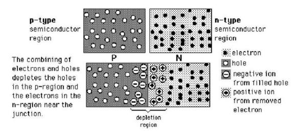
Filling a hole makes a negative ion and leaves behind a positive ion on the N side.
