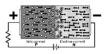
current through a PN junction. Bias voltage imparts sufficient energy to the free electrons so they overcome the barrier potential and move into the P region.
