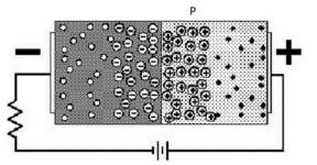
Reverse bias potential attracts the majority carriers away from the PN junction widening the depletion region. The potential across the depletion region is equal to the bias voltage. Reverse current can flow through the PN junction due to minority carriers. When a PN junction is reverse biased the energy hill increases.
