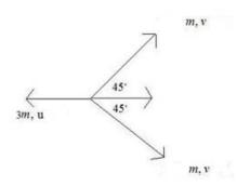
The initial moment of a bomb is zero. That's why vertical and horizontal components of final moment of a system are zero too. The horizontal components of final moment is
