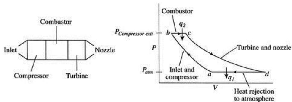
**Figure 1:** Sketch of the jet engine components and corresponding thermodynamic states
