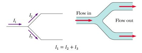
Kirchhoff's junction rule is an application of the principle of **conservation of electric charge**: current is flow of charge per time, and if current is constant, that which flows into a point in a circuit must equal that which flows out of it.
