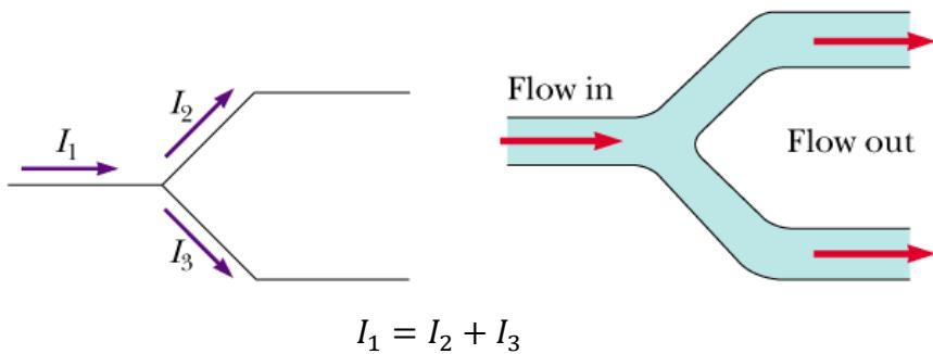
Kirchhoff's junction rule is an application of the principle of **conservation of electric charge**: current is flow of charge per time, and if current is constant, that which flows into a point in a circuit must equal that which flows out of it.
