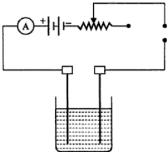
Electric current is passed for a known time  $t = 1 \text{ hour} = 3600 \text{ s}$ . The mass of silver deposited on the cathode is measured.
