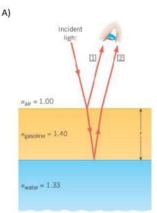
Because of reflection and refraction, two light waves enter the eye when light shines on a thin film of gasoline floating on a thick layer of water. Because of the extra distance traveled, there can be interference between the two waves.
