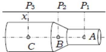
The magnetic field at 1, 2 and 3 is equal. To find magnetic field outside a thick conductor, the current may be assumed to flow along the axis. As points 1, 2, 3 are equidistant from the axis. So, magnetic field at these points is also equal.
