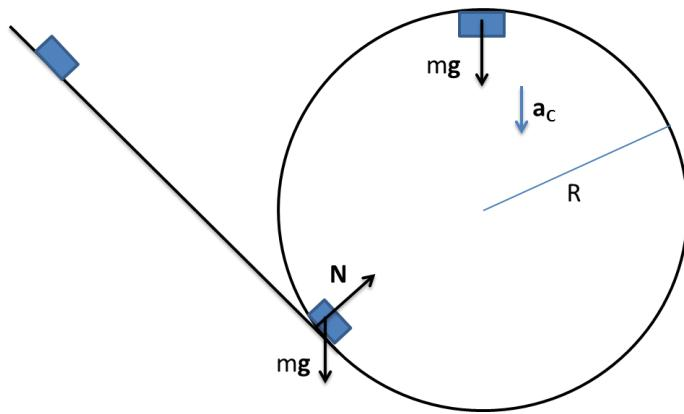
The necessary and sufficient condition for rider to remain in the loop is the normal force in the highest point is more or equal to zero:
