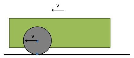
Let's move to the frame of reference, associated with the car. In this frame of reference car is in the state of rest and the bottom point of tires moves with velocity  $\mathbf{V}$  to the opposite direction:
