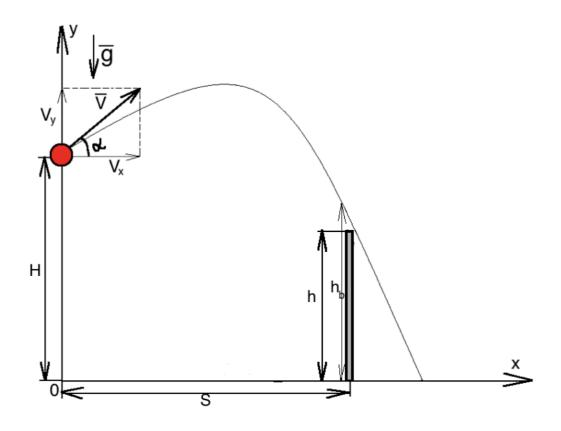
Equation of the motion for the ball, directed at angle  $\alpha$ : (t - time of the flight)  $V_x = V \cos \alpha$ ;  $V_y = V \sin \alpha$ ; x:  $S = V_x t = V t \cos \alpha$  $t = \frac{S}{V \cos \alpha}$  (1)
