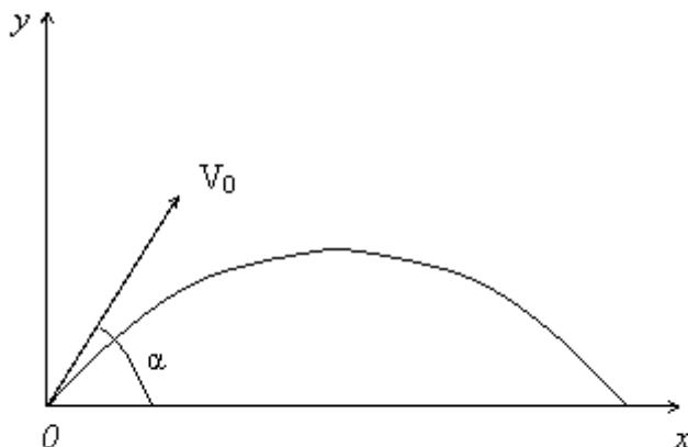
Fig. 1. Motion of body thrown at angle to the horizon.
