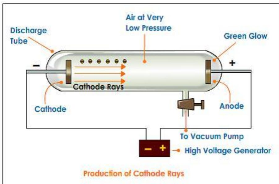
It was found that gases could not conduct electricity even when an electrical potential of about 10,000 volts was applied. But, it was discovered by William Crookes that gases could conduct electricity at low pressures. When, the pressures inside the discharge tube were reduced gradually, the following point was noted.
