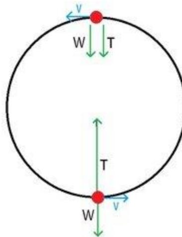
If you have a ball on the end of a string and you swing it in a vertical circle the "centripetal force" or the forces causing the acceleration will be a combination of the tension from the string and gravity.
