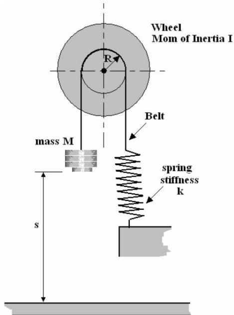
We suppose the mass is pulled downwards with a force  $F$ . This must overcome the inertia of the mass, the inertia of the drum and stretch the spring.
