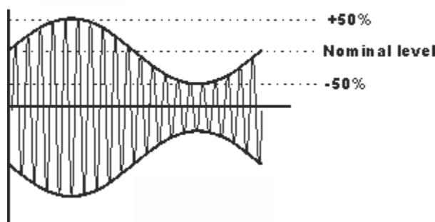
The amplitude modulation depth is
