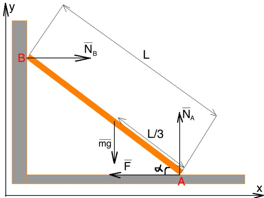
$\alpha = 30^\circ$  – angle which ladder makes with the wall
