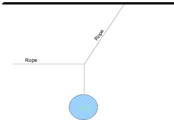
The object of our focus here is the knot where all the ropes converge. Draw a free-body diagram for the knot.
