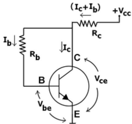
fig.2. collector-to-base bias
