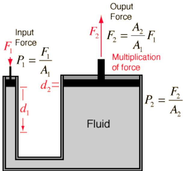
$$F_1 / \text{Area small piston} = F_2 / \text{Area of large piston}$$
