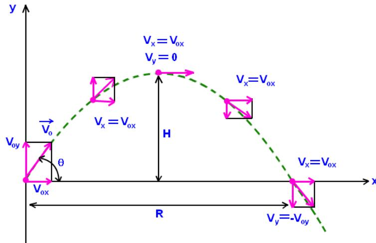
Equations related to trajectory motion (projectile motion) are given by
