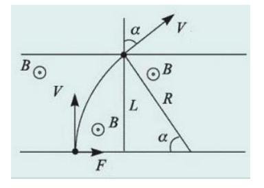
Magnetic force that acts on the each proton in the beam (q - charge of the proton):  $F = qVB \quad (1)$
