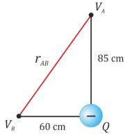
When the charge creating the field is positive, the voltage is positive; when the central charge is negative, the voltage is negative.
