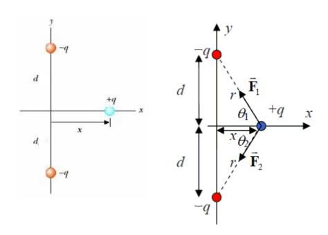
The net force on the q charge is  $\vec{F} = \overrightarrow{F_1} + \overrightarrow{F_2}$ . Since  $F_1 = F_2 = \frac{kq(-q)}{r^2} = -\frac{kq^2}{r^2}$ , with  $r = \sqrt{x^2 + d^2}$  and from the symmetry  $\theta_1 = \theta_2 = \theta$  so the y-components of  $\overrightarrow{F_1}$  and  $\overrightarrow{F_2}$  cancel. So the magnitude of  $\vec{F}$  is  $F = F_1 \cos \theta + F_2 \cos \theta$  with  $\cos \theta = \frac{x}{r}$ . Therefore
