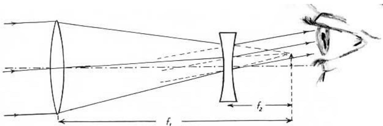
Objective is a convex lens of large focal length  $f_1$ ;
