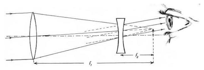
Objective is a convex lens of large focal length  $f_1$ ;
