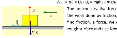
The nonconservative force in this problem is friction. To find the work done by friction, we need to know the friction. To find friction, a force, we draw a Free–Body Diagram at the rough surface and use Newton's Second Law.
