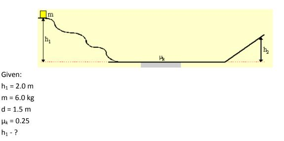
Since the problem involves a change of height and speed, we make use of the Generalized Work-Energy Theorem. Since the block's initial and final speeds are zero, we have
