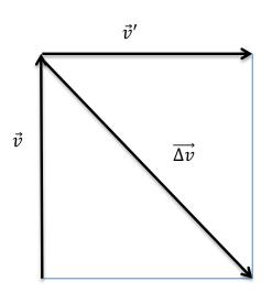
where  $\vec{v}$  is velocity directed to north,  $\vec{v'}$  is velocity directed to East,  $\overrightarrow{\Delta v}$  is change in velocity.
