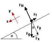
Here  $F_x$  is the force in the x direction,  $F_y$  is the force in the y direction,  $F_g$  is the force of gravity,  $F_N$  is the normal force and  $F_f$  is the force of friction. Finally,  $\theta$  is the angle of the slope (in our case,  $\theta = 14^\circ$ ).
