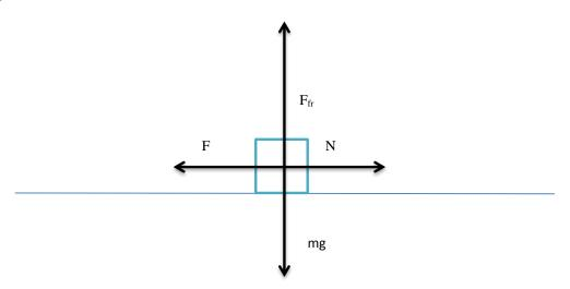
Where F – horizontal force with which man is pressing the pole, N – normal force
