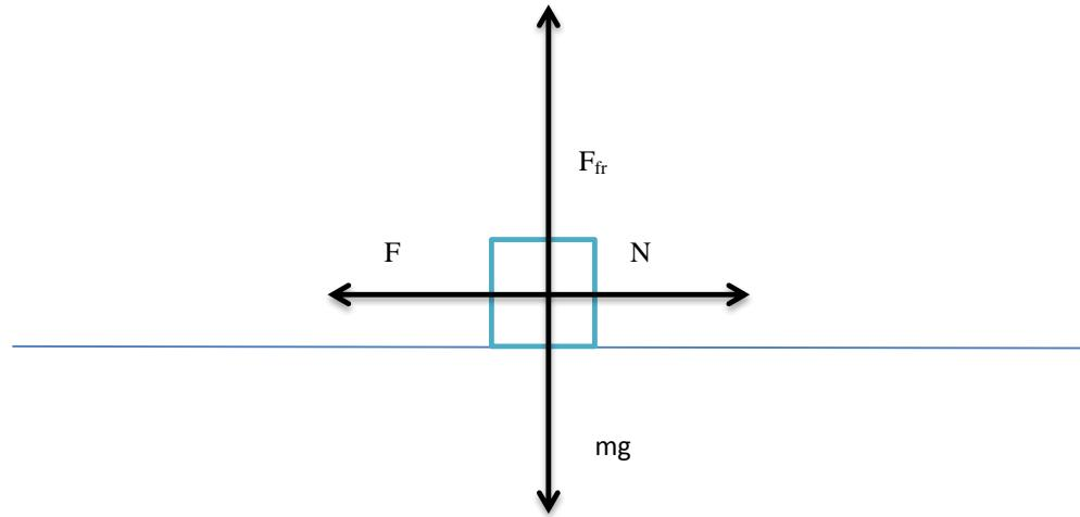
Where  $F$  – horizontal force with which man is pressing the pole,  $N$  – normal force
