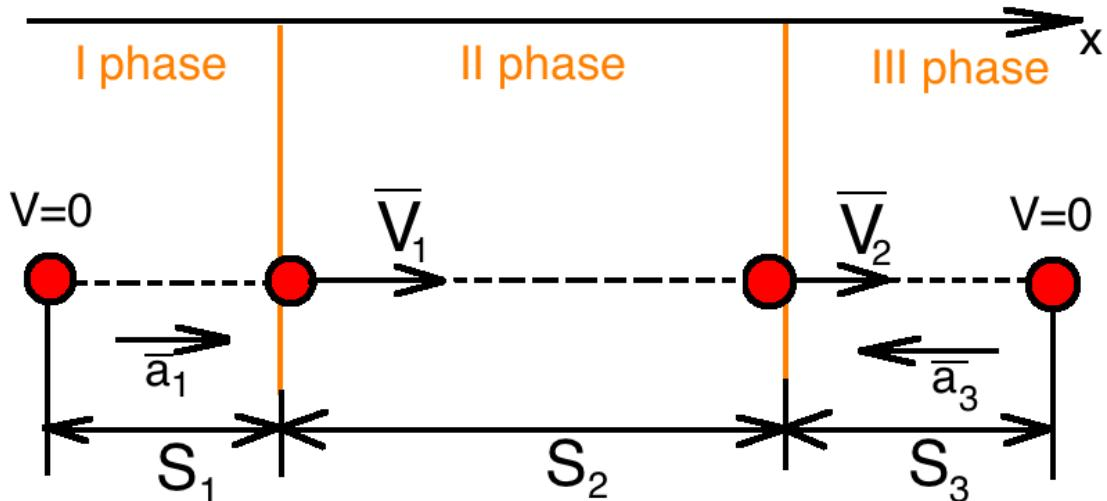
Assumption: to find the average speed we can break all path up into three phases: accelerating  $\rightarrow$  coasting  $\rightarrow$  decelerating.
