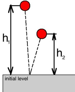
$E_1 = mgh_1$  – initial mechanical energy (potential energy at a height  $h_1$ );
