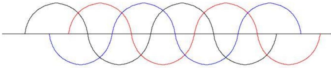
The strength of the magnetic field changes, as the current flow in the coils of wire around the stator poles change. Just as the current in the field windings rise and fall 120 electrical degrees apart, so does the resulting magnetic field on the pole face. In other words, when the magnetic polarity on pole 'A' reaches it's peak, 120 electrical degrees later pole 'B' will reach it's peak, and
