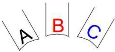
The stator windings are arranged on the stator poles in a way that results in magnetic flux lines that seem to rotate. In this example, the direction of rotation would be clockwise. Can you see that changing any two leads would result in counter-clockwise rotation?
