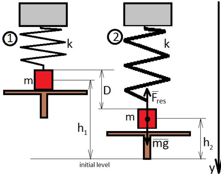
For the initial level of the system we will take the position of the board after the weight hanging on a spring,  $k$ - spring constant;
