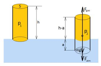
Mendeleev-Clapeyron equation for gas in the first and in the second case:
