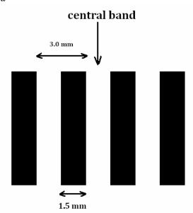
As it can be seen from a picture above, the spacing between interference fringes is equal to the  $\frac{3.0}{2} = 1.5 \ mm$
